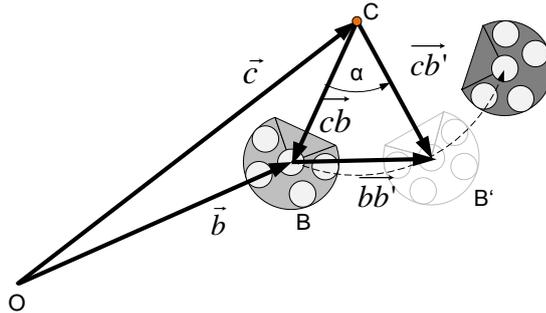
**Fig. 3.** How to move on a circular trajectory
