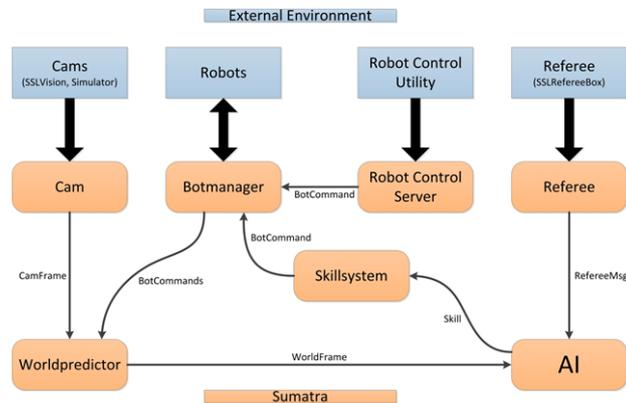
**Fig. 2.** Sumatra Architecture and its connection to the periphery
