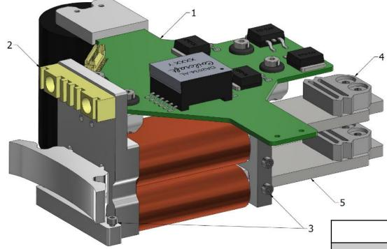
The kicker module consists of two plungers (5) made of aluminum and ferromagnetic steel. Two 3D printed flexible dampers absorb impact energy (4). Retraction springs are mounted on (3). The kicker board uses a line transformer and the LT3751 IC to charge two  $1800\mu$ F capacitors to up to 250V within two seconds.
