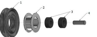
Two friction bearings (3) reduce vibration and wear on the bearing. A simple dowel pin (4) is used as an axis. Apart from the roller body all components are available off the shelf.
