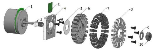
The usage of 65W motors makes it possible to use a direct drive and still have enough torque for good acceleration. The wheel can be fully removed by removing a single hex nut (10).
