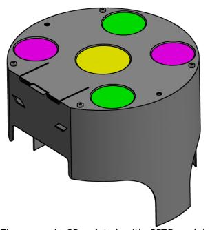
The cover is 3D printed with PETG and has a wall thickness of 1.2mm. It will be fully covered with a adhesive sticker containing logos and robot number. The cover and the sticker form a very robust compound material. While we expect the cover to crack eventually it will still be fully functional due to the sticker holding everything together. As the covers are 3D printed they are easy to replace in case of too many cracks.
