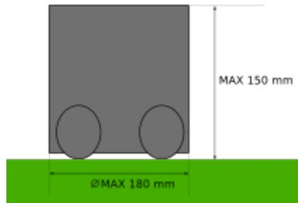
Figure 3: The maximum robot dimensions
